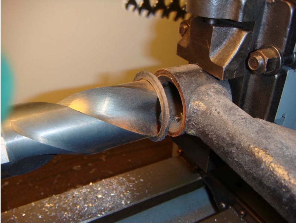
Figure 7 – The flange coming free on the drill bit.
