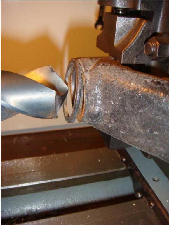
Figure 6 – The flange after being tapped with a punch
