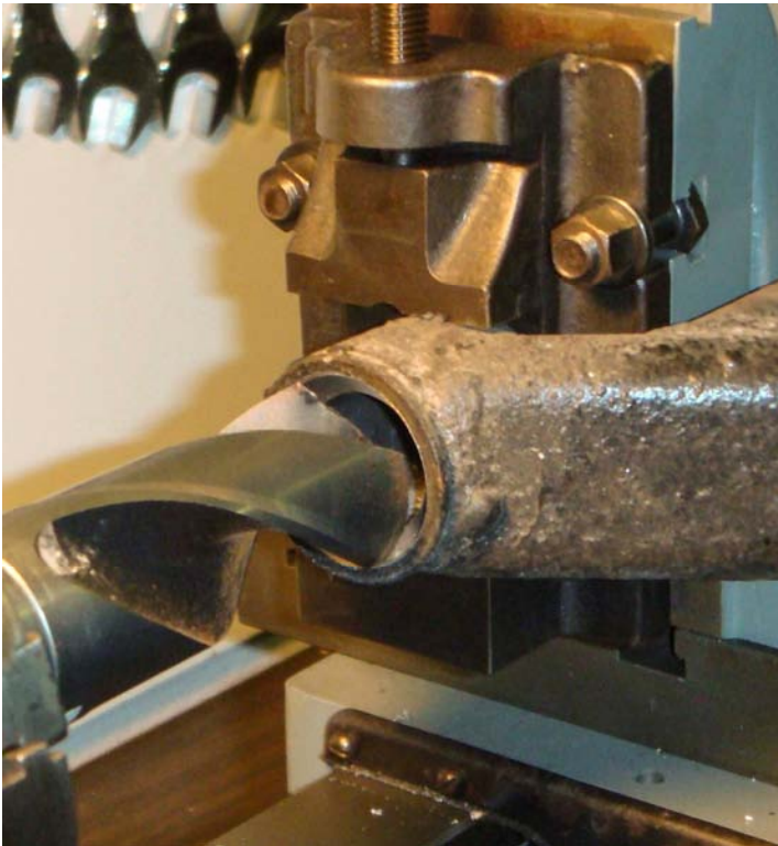
Figure 5 – Milling attachment vise set-up
