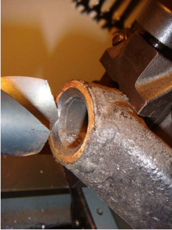
Figure 4 – First cuts into the sleeve
