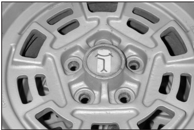
The 1971 two-slot wheel introduced profound changes. The center is identical, but the webbing has been widened slightly, and no longer reaches the top of the wheel center. The raised surfaces and the pentagon have now been given a softer, more rounded appearance
