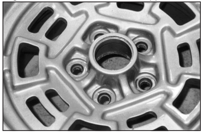
The 1972 Pre-L two-slot wheel changed yet again. The hub has been enlarged, requiring small reliefs to allow lug wrench clearance. The webbing has also been widened slightly, and the raised surfaces and the pentagon have now been raised from the face of the wheel and are slightly taller
