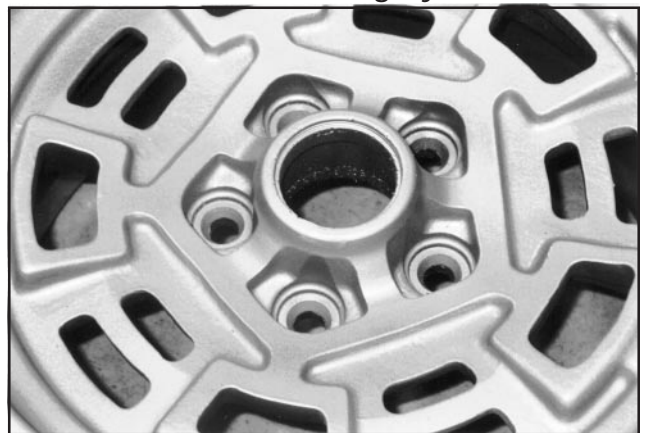
The later L-model wheel was almost identical to its immediate predecessor, but the wheel center has been fortified yet again, requiring even larger reliefs for lug wrench clearance. The webbing is wider and no longer tapers towards the center
