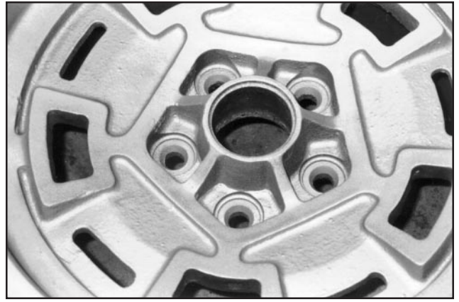
The one-slot wheel is identical to the three-slot wheel save for the lack of the two inner slots. The wheel center is rather modest, with narrow webbing connecting it with the pentagon. Both the pentagon and the raised surfaces containing the larger holes have a flat, machined appearance
