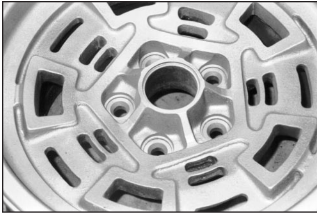
The three-slot wheel was never used on Panteras exported to the USA, and was only found on the very earliest European cars. Publicity photos of prototype Panteras show these wheels, but they were virtually never seen on cars sold to customers. The features are very sharp and crisp
