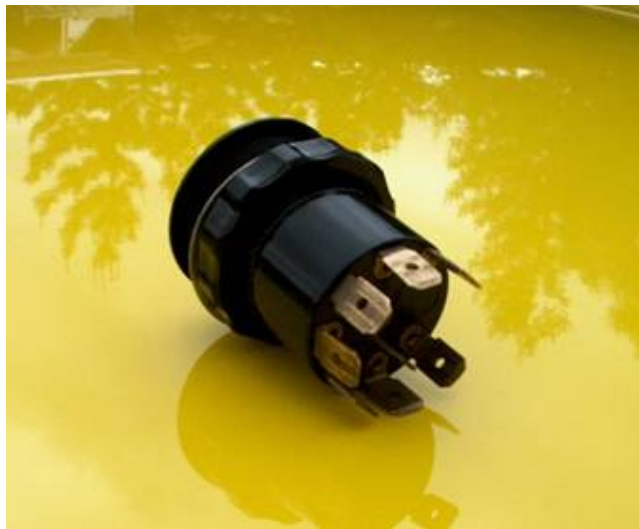
View of backside of switch removed from car.
