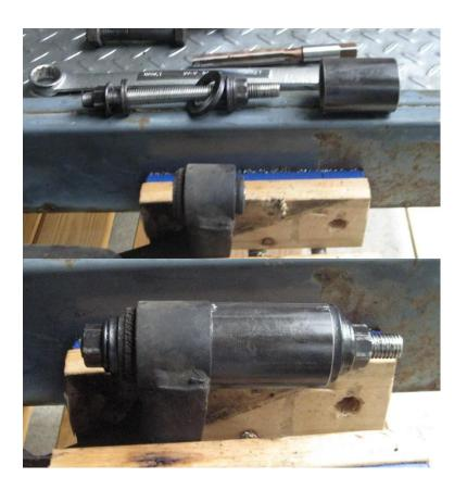
Initially the inner sleeve spool compresses the rubber and given my bushings had swollen and cracked, a doughnut is sheared off before the inner spool starts pushing on the outer sleeve. the "break away" torque required a good one hand push with long box end wrench, and after that it was just a matter of wrenching the old bushing its length to free the a arm. A deep socket on a ¼" drive was handy incase the stud started spinning the far nut.
