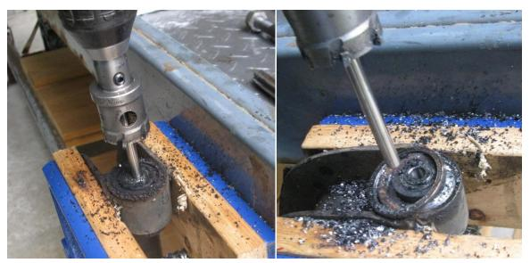
Again from Wal-Mart's online, I got M12X140mm studs, heavy washers and nuts. Applied thread lube and assembled the receiver to pull the bushing from the sleeve
