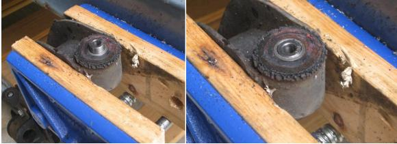
A 30MM hole drill, also from Wal-Mart's online, was modified by removing its 6mm pilot drill bit and a¼" drill blank installed (guess where it was from!). The first cutting removes the bushing's rubber and then starts cutting into the flange. I intentionally took things slow here, to ensure I stayed fairly centered in the ARM and just cut till the flange spun off.
