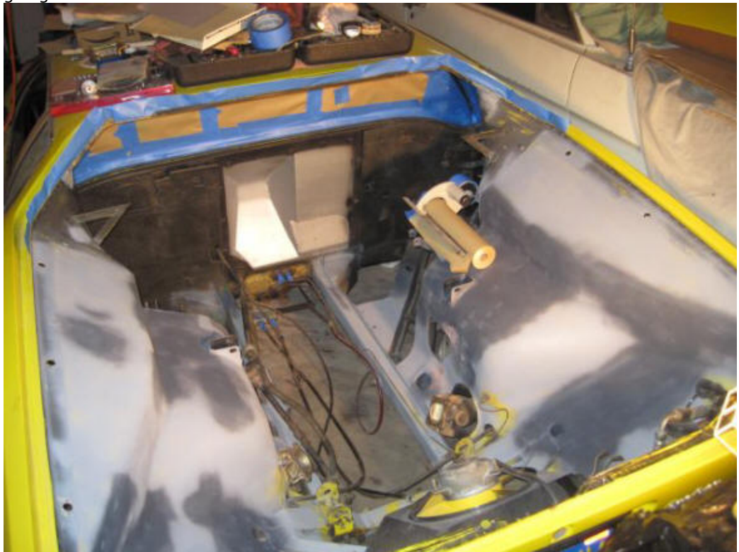
Masking to repaint the flat black areas at the front of the engine compartment and under the roof, as well as the inside-rear tail light panel.
