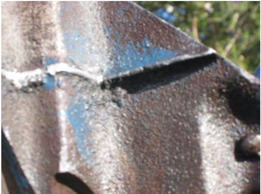
De-burred the block - Smoothed casting flash for a cleaner appearance - not that anyone will be able to see this in the Pantera.
