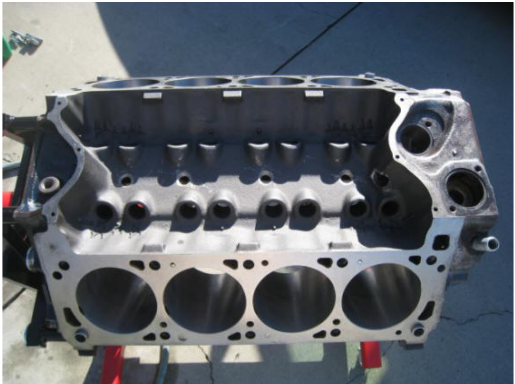
De-burred the block - Smoothed casting flash for a cleaner appearance - not that anyone will be able to see this in the Pantera.
