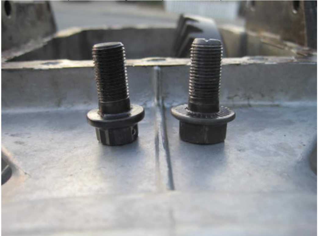
New ARP bolt compared to the original bolt (ARP bolt on left).
