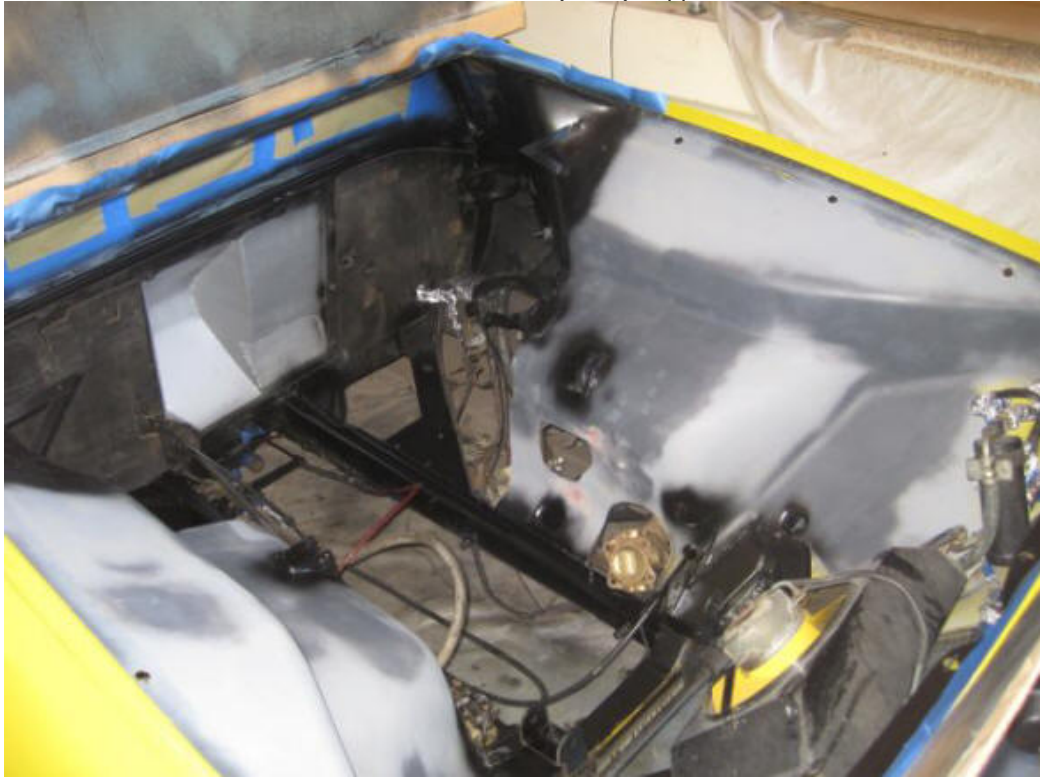
First coat of Eastwood Chassis Black Extreme (satin). Applied two coats.
