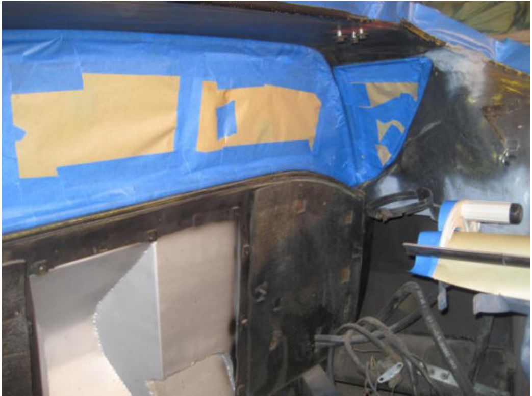
First coat of Eastwood Chassis Black Extreme (satin). Applied two coats.
