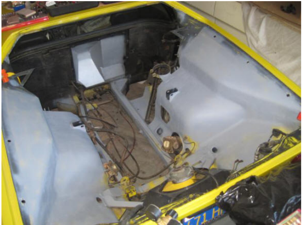
Sandable filler primer - I really shouldn't have put this much effort into the finish since it's going to be covered with truck bed-liner.
