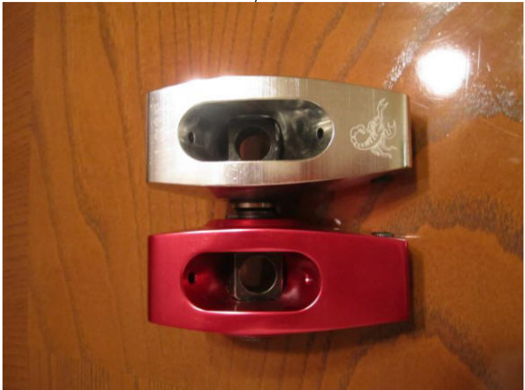
Interesting to compare the size differences. Both are 1.73 ratio 351C rocker arms. The casting on the ProComps is beautiful, but Scorpion is a name I know and trust. Plus, the Scorpion rocker arms come with a lifetime warranty.
