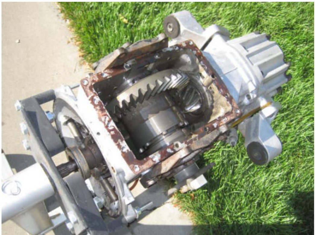
I used these pieces of steel track to lock against the half-shaft bolts in the axle flanges to keep the ring gear from turing while I broke the bolts free.
