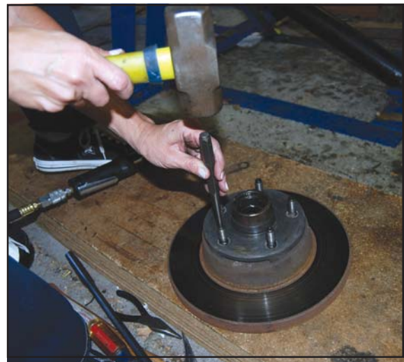
A BFH and a pointed punch are used to drive the studs out of the stock rotor/hub assembly, although a press would be preferable
