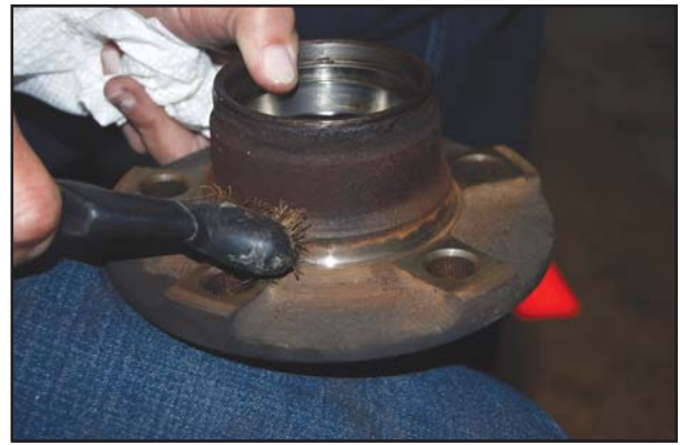
The area where the inside of the rotor seats against the hub needs to be thoroughly cleaned to ensure the discs rrrn perfectly true, or else the brake pedal will pulse
