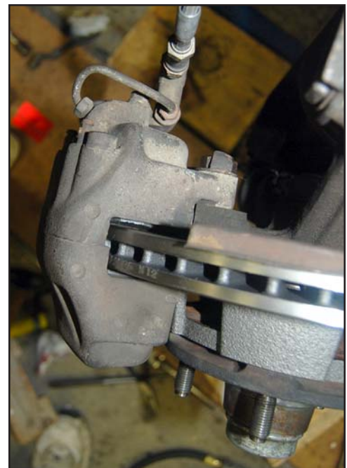
The end result—beautiful vented rotors which fit absolutely perfectly, deliver a noticeable improvement in consistant stopping power under aggressive use, at a fraction of the cost of the alternatives
