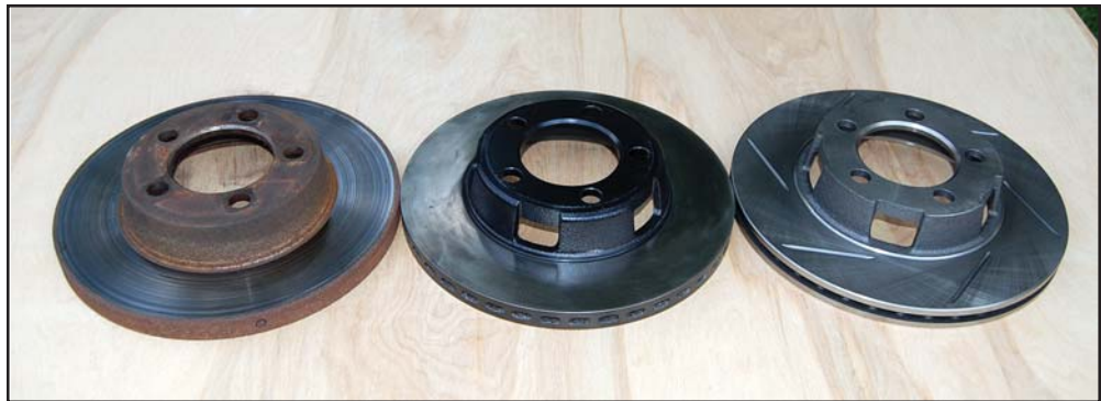
Left to right, stock solid Pantera rotor, rare Euro GTS vented rotor, and new '65-'67 Ford Mustang rotor. The dimensional differences are thankfully trivial
