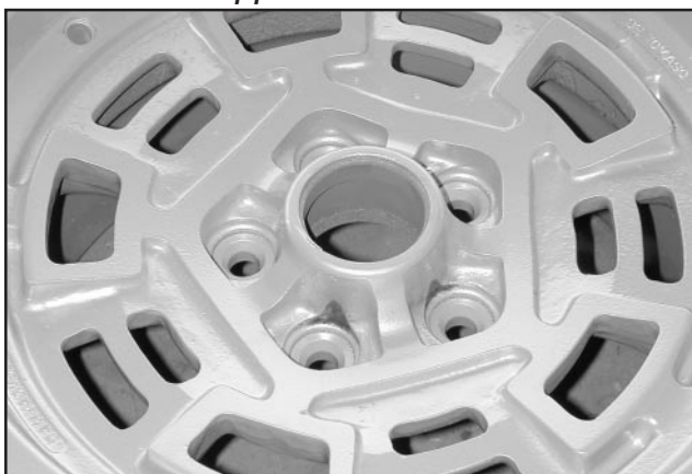
The first L-model wheel brought a return to some original design themes. The hub was strengthened even further, and the webbing was increased in size yet again. The pentagon is now flat, but the raised surfaces still retain a rounded contour
