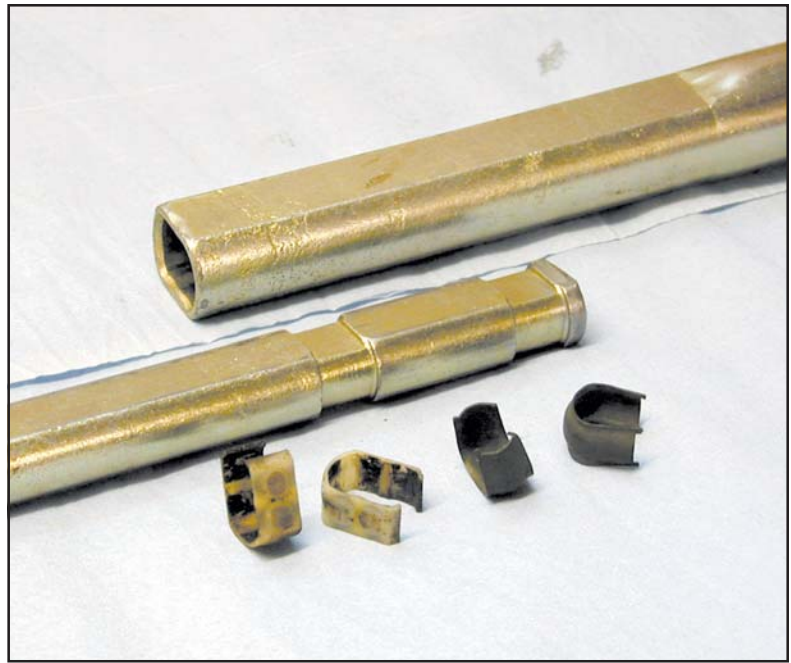
The male and female slider portions of the steering shaft system (these have been freshly cad-plated), along with the original nylon bushings (the two circular raised spots on each side are almost entirely worn away), and Wilkinson's stamped steel replacements
