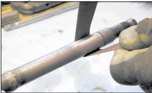
It is important to sand or polish the steering shaft smooth, so the bearing can spin freely upon it
